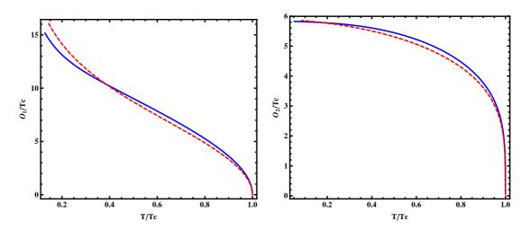
Figure 2.14: Condensate of the scalar operator as a function of the temperature for  $\mathcal{O}_{-}$  (left) e  $\mathcal{O}_{+}$  (right). Straight blue line is  $f(\phi) = \cosh(\phi)$  and dashed red line is  $f(\phi) = 1 + \phi^{2}/2$ . In both cases the potential is  $L^{2}V(\phi) = -6 - \phi^{2}$ . For the two operators we have  $T_{c} \sim 0.182\sqrt{\rho}$  and  $T_{c} \sim 0.135\sqrt{\rho}$  respectively.
