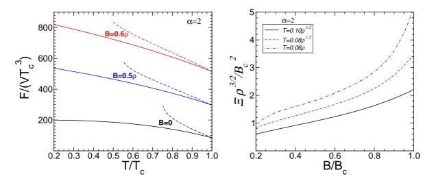
Figure 3.3: Left panel: free energy for DDBHs (straight lines) and for AdS-RN black holes (dashed lines) as a function of the temperature for selected values of the magnetic field. Right panel: normalized magnetic susceptibility for DDBHs as a function of the magnetic field. We use  $f(\phi) = \cosh(2\phi)$ .
