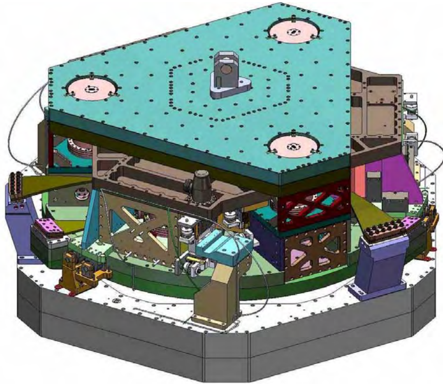
Figure 5.25: Rendering of redesigned BSC ISI. The ISI is rigidly fixed to HEPI and provides two stages of active isolation for the chamber’s optical table.
