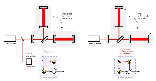
Figure 3.1: Left: a traditional 'balanced photodiode' homodyne detection arrangement. Right: DC readout with two photodiodes.
