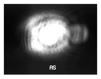
Figure 4.1: Image of the beam spot at the L1 output port taken using a CCD camera. This image is saturated in the central portion but emphasizes the spurious higher order modes surrounding the fundamental Gaussian, including contributions from both the carrier and the 25 MHz sidebands.
