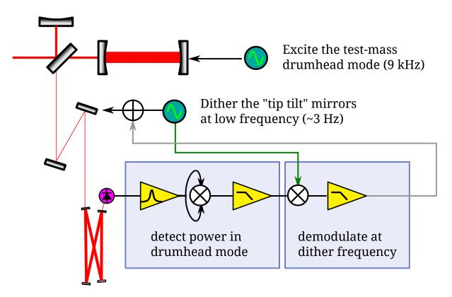
Figure 4.6: The 'Drumhead dither' OMC alignment system.
