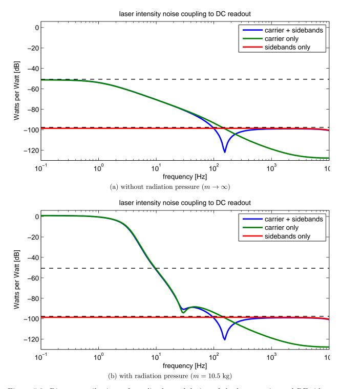
Figure 5.3: Direct contributions of amplitude modulation of the laser carrier and RF side-bands to DC readout, in the absence of radiation pressure. The carrier contribution is shaped by the coupled cavity pole. The RF contribution is due to residual off-resonance transmission through the OMC. Interference between the two coupling mechanisms creates a dip in the total coupling at the crossover frequency.
