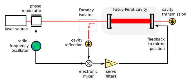
Figure 2.5: In the basic Pound-Drever-Hall setup, a phase modulator is used to produce RF sidebands well outside of the cavity bandwidth. The light reflected from the cavity is incident on a photodiode, the signal from which is demodulated to produce an error signal indicating the mismatch between cavity length and laser carrier frequency. Through feedback, the cavity can be 'locked' to the resonance. The technique can be generalized to sense and control much more complex interferometers.
