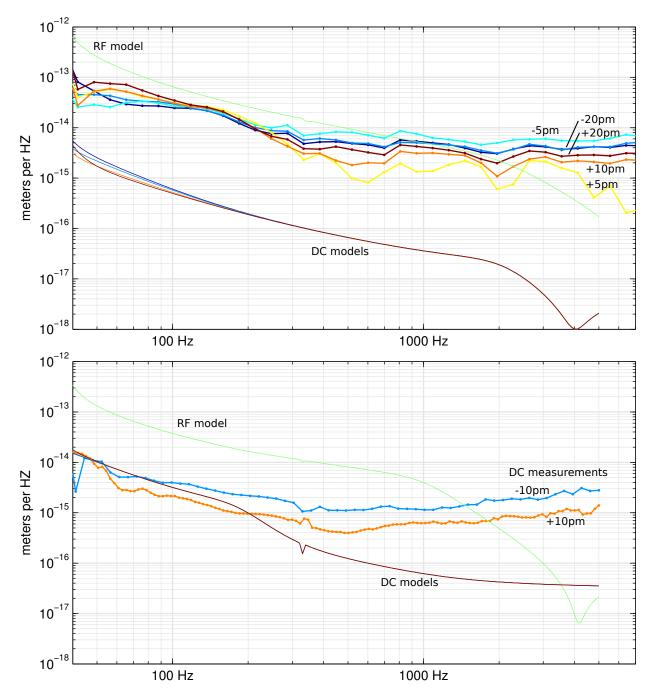
Figure 5.5: Laser frequency noise coupling to DARM
