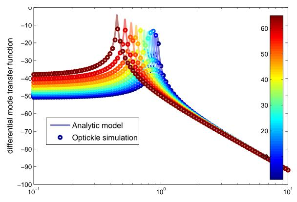
Figure D.1: The optical spring effect: As a cavity is detuned from resonance, the resonance of the differential mode deceases. This figure compares the results of a numerical (Optickle) model with analytic results. The units of the y-axis are  $20 \log_{10}(\text{displacement/force})$ ; the x-axis is Hz; color indicates cavity detuning in picometers.
