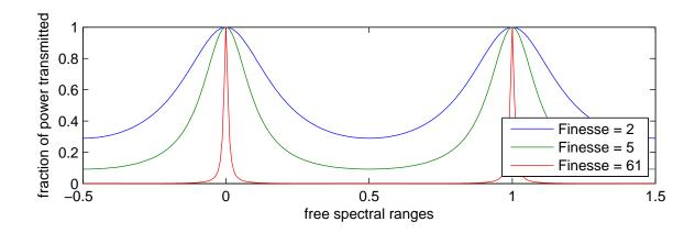
Figure C.3: Power transmission coefficients for three critically-coupled cavities.
