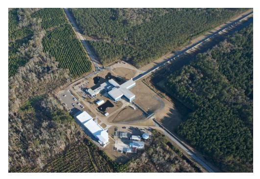
Figure 1.3: Aerial photo of the LIGO Livingston Observatory, containing the L1 detector. The main building in the center of the photo contains the beamsplitter; the two 4 km arms reach out to the right of the photo. Photo by Greg Grabeel and the author.
