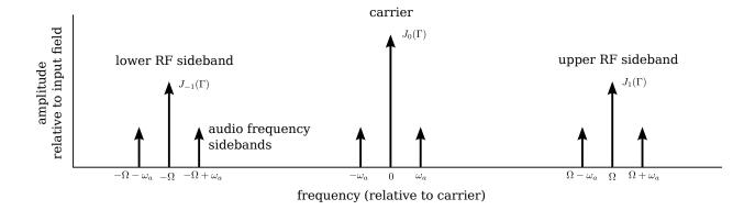
Figure 5.2: Schematic diagram of the laser carrier and RF sidebands, and their associated audio-frequency sidebands.
