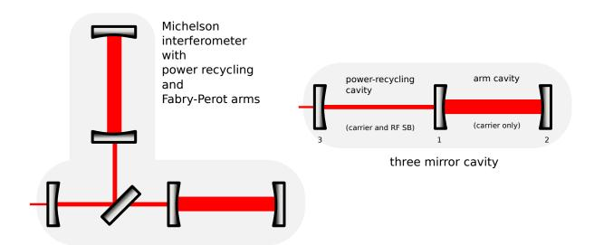
Figure 2.3: It is sometimes convenient to condense the two arms of the Power-Recycled Fabry-Perot Michelson interferometer into a single 'virtual arm' for the purpose of analysis.
