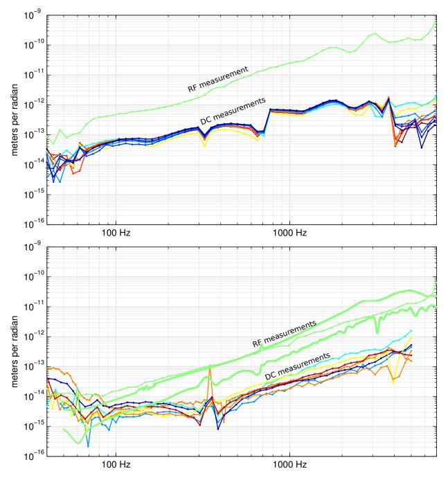
Figure 5.7: Oscillator phase noise coupling to DARM.
