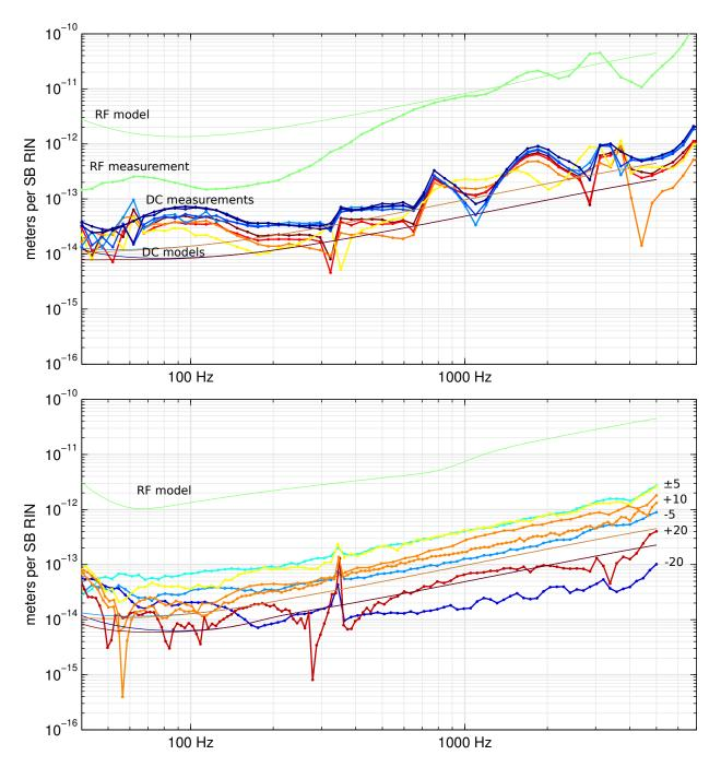
Figure 5.6: Oscillator amplitude noise coupling to DARM
