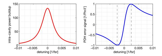
Figure 2.6: (a) Power buildup inside a resonant cavity relative to the incident power, as a function of cavity detuning (deviation from resonance). (b) The Pound-Drever-Hall error signal as as a function of detuning (in watts relative to the incident power and the modulation depth). The dashed lines indicate the region in which PDH provides a usable error signal with which to lock the cavity. The cavity modeled here has parameters similar to the initial LIGO arm cavities.
