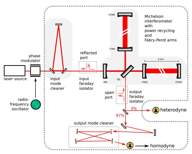
Figure 3.4: Enhanced LIGO interferometer layout (not to scale). The dotted line represents the vacuum enclosure.
