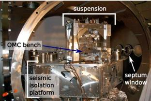
(b) Photograph of installed OMC and suspension
