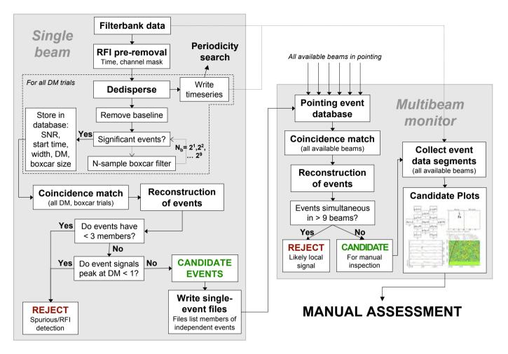
event in the pointing not tagged as interference periodicity simultaneously, distributed onto Each of up to 13 "single beam" processes associated with one multibeam pointing are run on multiple-beam occurrence, search results for that beam. diagrammatic representation of the HTRU collecting single-pulse several and producing single-event diagnostic plots for each The multibeam monitor tracks the status of the performing interference excision Survey's single-pulse pipeline.
