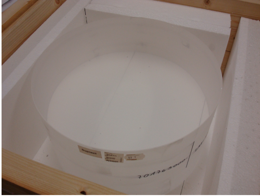
Figure 1.12: Input mirror blank (35 cm diameter, 20 cm thickness).
