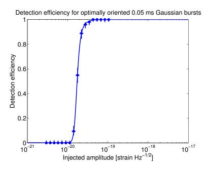
Figure 7.24: The detection efficiency as a function of characteristic strain amplitude ||h|| for optimally oriented populations of simple Gaussian bursts with duration  $\sigma_t$  of 0.05 milliseconds. The detection efficiency is shown at a detection threshold corresponding to the coherent normalized energy of the most significant foreground event.
