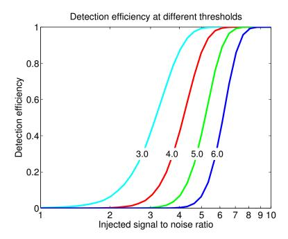
**Figure 5.5:** Theoretically predicted detection efficiency curves for well localized bursts in the presence of stationary white noise. The detection efficiency at a particular injected signal to noise ratio is determined by identifying the fraction of events that exceed a specified threshold on the observed signal to noise ratio. Here, we have considered observed signal to noise ratio thresholds of 3, 4, 5, and 6.
