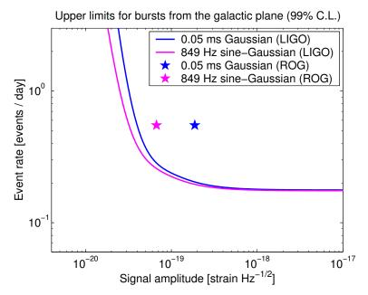
Figure 7.31: Upper bounds on the rate gravitational-wave bursts in the galactic plane. Upper limits are shown at a 99 percent confidence level for simple Gaussian bursts with a duration  $\sigma_t$  of 0.05 milliseconds (blue) and sinusoidal Gaussian bursts with a central frequency of 849 Hz and a Q of 12.7 (magenta), and compared with the postulated excess of events reported by the ROG collaboration[13, 14].
