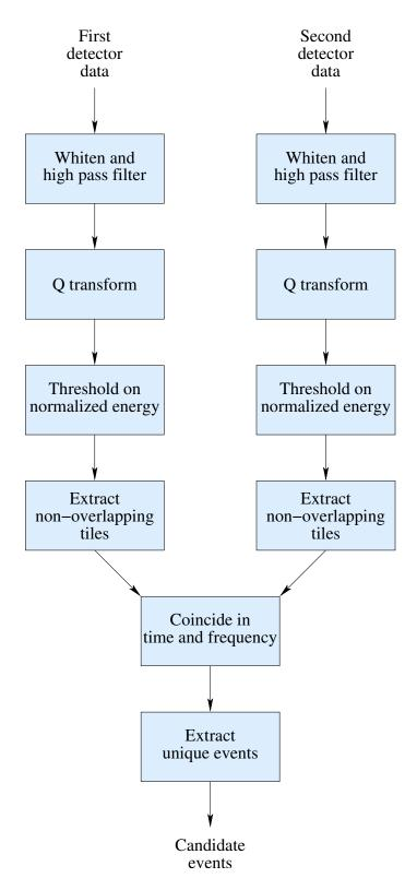
Figure 5.10: The proposed end-to-end analysis pipeline for the identification of coincident candidate gravitational-wave bursts in data from multiple interferometric detectors.
