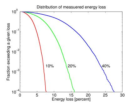
**Figure 6.1:** The cumulative distribution of the fractional energy loss incurred by arbitrary well localized bursts in the targeted signal space as a result of mismatch with the nearest measurement tile. The resulting distributions are clearly consistent with the requested worst case fractional energy losses of 10 (red), 20 (green), and 40 (blue) percent. In all cases, this worst case loss is never exceed in 10<sup>4</sup> measurements.
