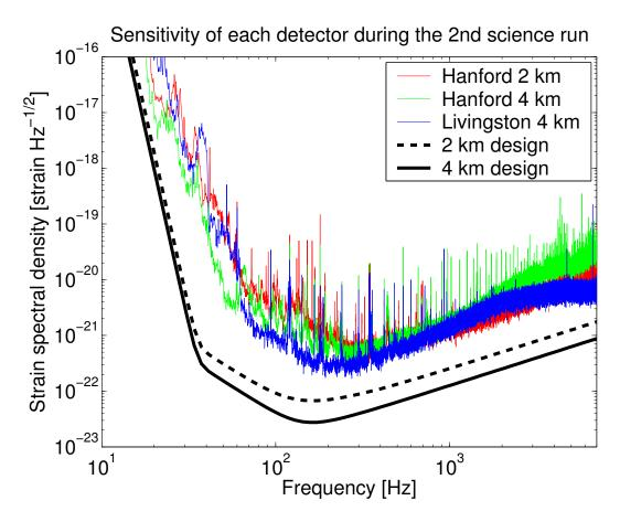
**Figure 2.7a:** The best sensitivity achieved by the Hanford 4km, Hanford 2km, and Livingston 4km detectors during the second LIGO science run are compared with the LIGO design sensitivity for 2 km and 4 km detectors. The definition of strain spectral density used to characterize the detector sensitivity is described in more detail in section 3.3.1 and is the same quantity used to characterize detector sensitivity in Figure 2.3.
