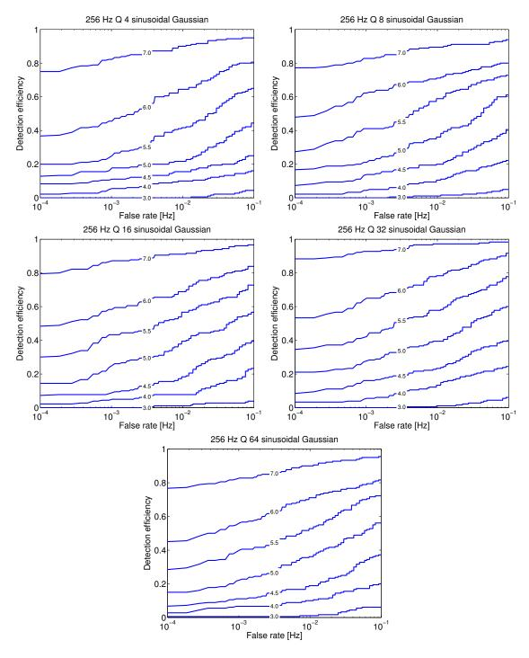
**Figure 6.7c:** Receiver operating characteristics of the single detector Q pipeline applied to 256 Hz sinusoidal Gaussian gravitational-wave bursts with Qs of 4, 8, 16, 32, and 64 injected into simulated detector noise at matched filter signal to noise ratios of 3.0, 4.0, 4.5, 5.0, 5.5, 6.0, and 7.0 as defined by Equation 3.32.
