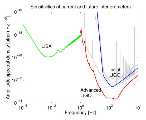
**Figure 2.8:** The design sensitivity of existing and future interferometric detectors. The initial design sensitivity of the 4 km LIGO detectors is compared with that of the planned second generation of LIGO detectors as well as the planned space-based interferometer LISA. For reference, we also show (in gray) the design sensitivities of the 2 km LIGO detector as well as the GEO600 and Virgo detectors (the lower of the three).
