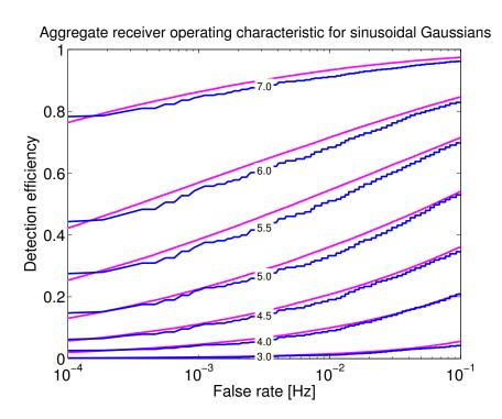
**Figure 6.8:** Aggregate receiver operating characteristic for all sinusoidal Gaussian waveforms. Each curve represents one value of injected signal to noise ratio. The empirically observed receiver operating characteristic (blue) shows reasonably good agreement with the theoretically predicted performance from Figure 5.7, which is also reproduced here (magenta) for comparison.
