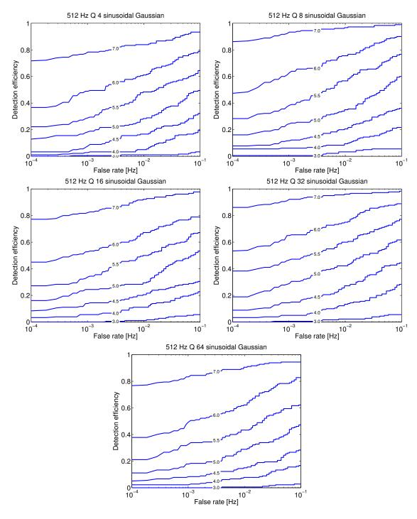
**Figure 6.7d:** Receiver operating characteristics of the single detector Q pipeline applied to 512 Hz sinusoidal Gaussian gravitational-wave bursts with Qs of 4, 8, 16, 32, and 64 injected into simulated detector noise at matched filter signal to noise ratios of 3.0, 4.0, 4.5, 5.0, 5.5, 6.0, and 7.0 as defined by Equation 3.32.
