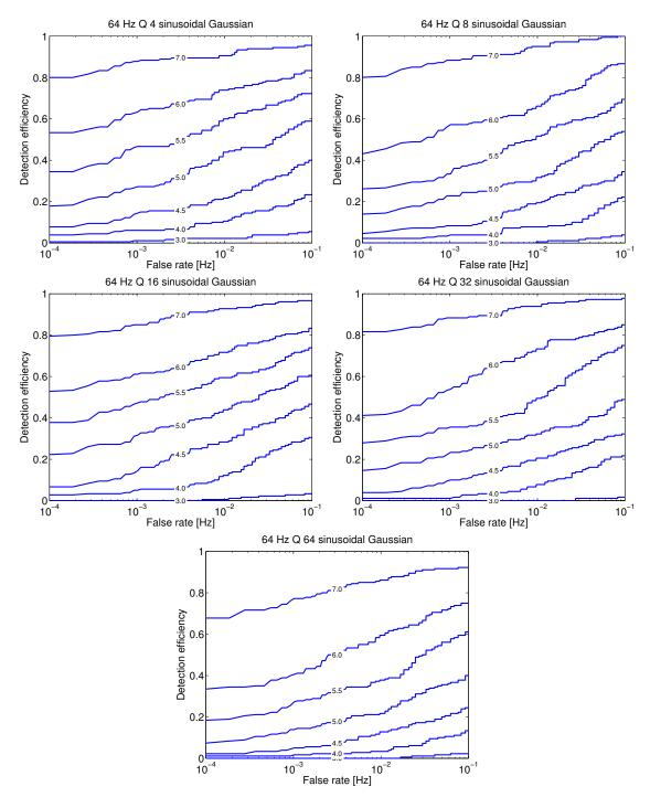
**Figure 6.7a:** Receiver operating characteristics of the single detector Q pipeline applied to 64 Hz sinusoidal Gaussian gravitational-wave bursts with Qs of 4, 8, 16, 32, and 64 injected into simulated detector noise at matched filter signal to noise ratios of 3.0, 4.0, 4.5, 5.0, 5.5, 6.0, and 7.0 as defined by Equation 3.32.
