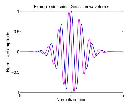
**Figure 3.1:** Example time-domain waveforms of a sinusoidal Gaussian burst with a central frequency of 1 Hz and quality factor Q of 10. Both even (blue) and odd (magenta) symmetric time-domain waveforms are shown, corresponding to the real and imaginary part of the complex valued waveforms given by Equation 3.11a and Equation 3.11b. Both waveforms are normalized to unity ||h||.
