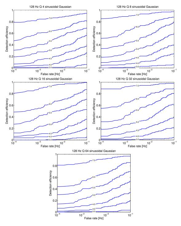
**Figure 6.7b:** Receiver operating characteristics of the single detector Q pipeline applied to 128 Hz sinusoidal Gaussian gravitational-wave bursts with Qs of 4, 8, 16, 32, and 64 injected into simulated detector noise at matched filter signal to noise ratios of 3.0, 4.0, 4.5, 5.0, 5.5, 6.0, and 7.0 as defined by Equation 3.32.
