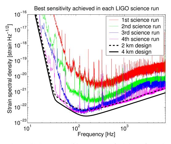
**Figure 2.7b:** The progression of detector sensitivity for the best performing detector during the first four LIGO science runs are compared with the LIGO design sensitivity for 2 km and 4 km detectors. The definition of strain spectral density used to characterize the detector sensitivity is described in more detail in section 3.3.1 and is the same quantity used to characterize detector sensitivity in Figure 2.3.
