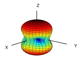
**Figure 2.5:** The angular response of interferometric gravitational wave detectors to gravitational waves with random linear polarization. Here the X and Y axes correspond to the orthogonal arms of an interferometric detector. The response has a maximum value of  $2/\pi$  for sources at the zenith of the detector and exhibits nulls for gravitational waves that are incident in the plane of the detector at 45 degree angles to the interferometer arms.
