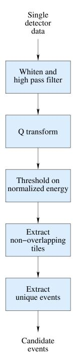
**Figure 5.9:** The proposed end-to-end analysis pipeline for the identification of candidate gravitational-wave bursts in data from a single interferometric detector. The same analysis pipeline is also applicable to the detection of statistically significant events in both environmental and auxiliary detector channels. This permits a test for environmental disturbances or pathological detector behavior in order to exclude events of non-gravitational-wave origin.
