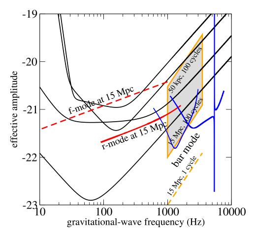
**Figure 2.14:** The gravitational wave signal amplitudes associated with neutron star instabilities are compared with the design sensitivities of current and future interferometric gravitational wave observatories. This figure has been reproduced from reference [19].
