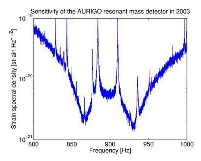
Figure 2.3: Strain spectral density for the AURIGA resonant mass detector at the same time as the second LIGO science run in December of 2003. The definition of strain spectral density used to characterize the detector sensitivity is described in more detail in section 3.3.1 and is the same quantity used to identify the sensitivity of interferometric detectors in Figure 2.7a and Figure 2.7b. The data for this figure is taken from Figure 1 of reference [32].
