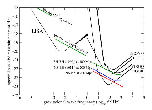
**Figure 2.11:** The expected signal amplitudes from the coalescence of binary compact objects of various masses are compared with the design sensitivities of current and future interferometric gravitational wave observatories. This figure has been reproduced from reference [19].
