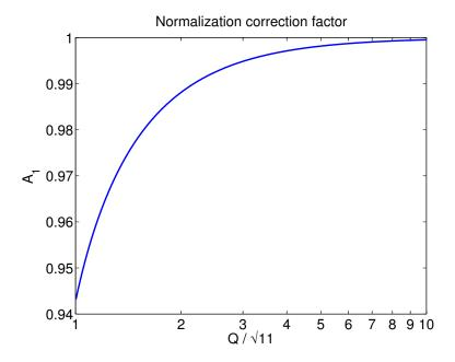
Figure 5.3: The necessary Q dependent normalization correction factor to allow for a complete accounting of the energy of non-localized bursts. Note that the correction is only marginally important at the minimum permissible Q, where the greatest frequency-domain overlap between tiles occurs. For larger values of Q, the correction factor quickly becomes negligible.
