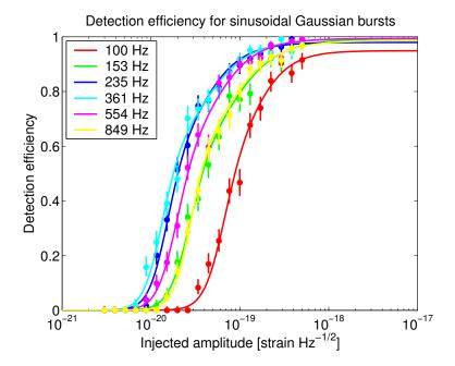
**Figure 7.15:** The detection efficiency as a function of characteristic strain amplitude ||h|| for isotropic populations of sinusoidal Gaussian bursts. Detection efficiencies are shown for bursts with a Q of 12.7 and central frequency  $\phi$  ranging from 100 to 849 Hz at a detection threshold corresponding to the coherent normalized energy of the most significant foreground event.
