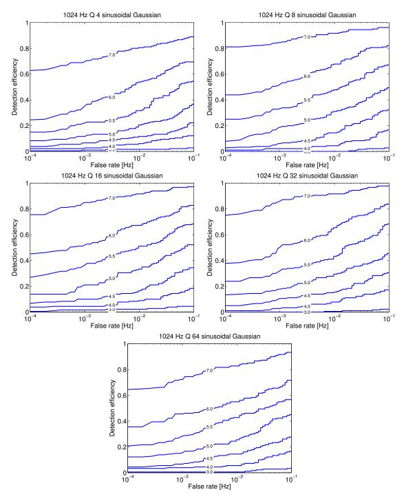
**Figure 6.7e:** Receiver operating characteristics of the single detector Q pipeline applied to 1024 Hz sinusoidal Gaussian gravitational-wave bursts with Qs of 4, 8, 16, 32, and 64 injected into simulated detector noise at matched filter signal to noise ratios of 3.0, 4.0, 4.5, 5.0, 5.5, 6.0, and 7.0 as defined by Equation 3.32.
