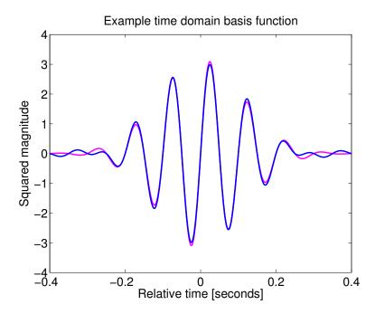
Figure 5.2: Example time-domain basis functions for both a Gaussian window (magenta) and bisquare window (blue). For comparison, both basis functions correspond to a time-frequency tile with a central frequency of 10 Hz and a bandwidth of 1 Hz, resulting in a Q of 10 as defined by Equation 3.6b, Equation 3.7b, and Equation 3.8. In addition, both are normalized such that the integral of their squared magnitude is unity.
