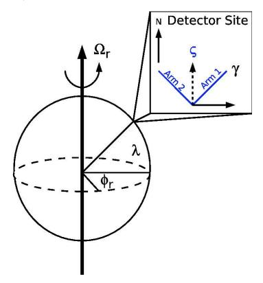
Figure 6-1: Diagram of a Interferometer located on the Earth's surface.  $\Omega_r$  is the Earth's rotation rate,  $\lambda$  is the latitude, and  $\phi_r$  is a reference phase which defines the position of the Earth in its diurnal motion at t=0. The inset shows a pair of interferometer arms as if looked down on from above. The angle  $\zeta$  is the angle between the arms (90° in the case of LIGO) while  $\gamma$  is the angle between East and the arm bisector.
