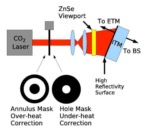
Figure 2-2: A schematic of the Thermal Compensation System (TCS). This was installed on both ITMs on all 3 LIGO interferometers. It is made up of a 10.6  $\mu$ m CO<sub>2</sub> laser, a set of interchangable masks, and a series of projection optics that produce an image of the mask on the optic.
